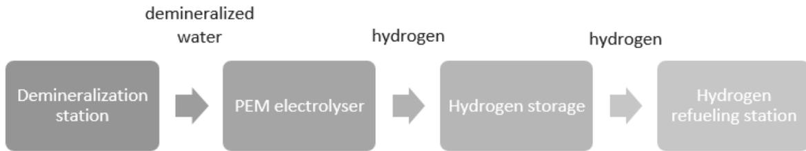
Picture 2. Installation for refuelling buses with hydrogen diagram
